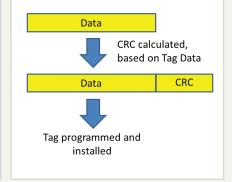
The tag's data and CRC code are read by the Tracklink III reader, which repeats the same calculation on (just) the data. The read and re-calculated CRC codes should of course be identical; thus validating the integrity and therefore validity of the read data.
