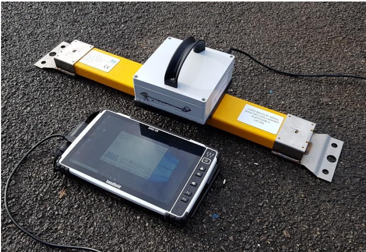
HSD2300/095 Programmer/Tester being used to program a HSD2300/090 beacon
