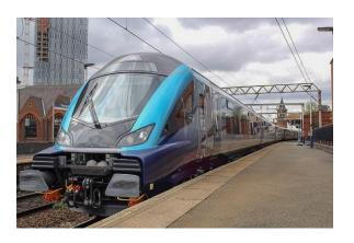
MK5A Coaches – Nova 3, Tracklink III® readers and EKE ASDO controller fitted to 13 x 5 coach sets hauled by Class 68 Locos. Used on TransPennine Express routes.
