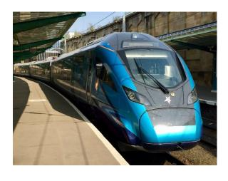
Class 397 EMU – Nova 2, Tracklink III® readers and EKE ASDO controller fitted to 12 x 5 car trains.
