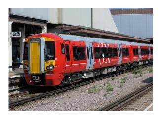
Class 387/2 EMU, Tracklink II® receivers fitted to 27 x 4 car trains. Tracklink II® beacons installed on Brighton & Gatwick Express routes.
