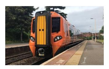
Class 196 DMU, Tracklink III® readers and EKE ASDO controller fitted to 12 x 2 car trains and 14 x 4 car trains. Used on West Midlands Trains..
