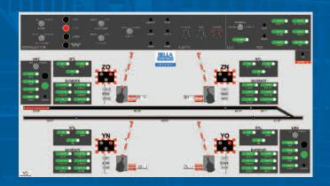
SELLA CONTROLS, in partnership with signalling designers has developed a COTS based Safety PLC solution for the provision of Level Crossing Control and the replacement of Simple Relay Interlocking Applications. Its solution architecture is based on a modern design using industry standard practices and the proven HIMatrix safety product suite.
