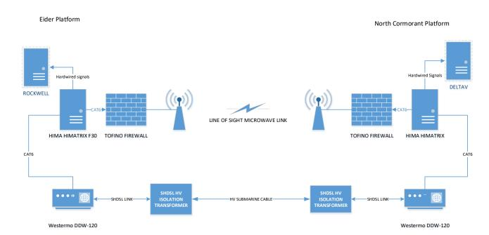
The examples above show that other media can be used such as fibre or even HV submarine cable.
